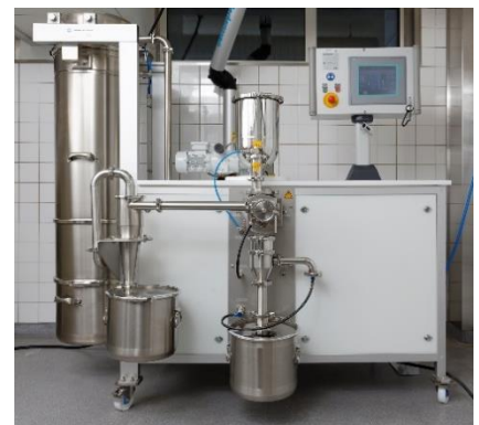
Figure 3. Air classifier used in protein enrichment.
